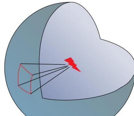
Figure 1: Example of incident energy projected onto a 1  $\text{cm}^2$  surface
