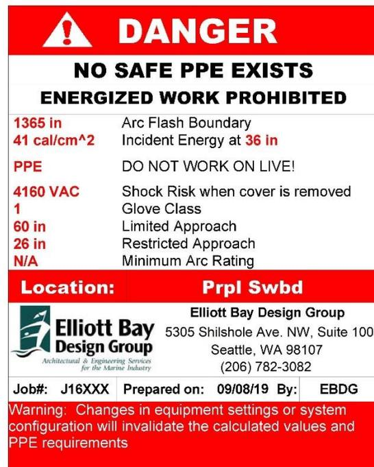
Figure 3: Example of an arc flash label
