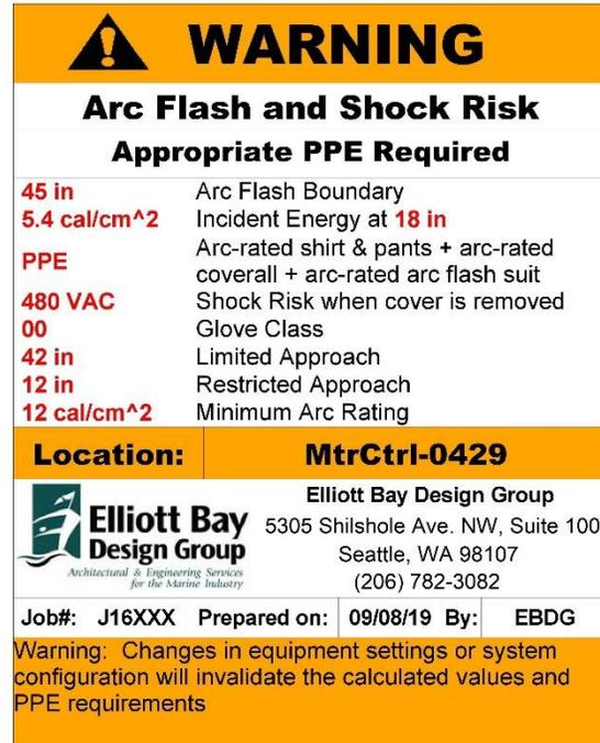
Figure 2: Example of an arc flash label
