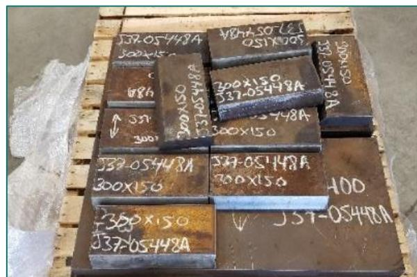
*Prepped Test Assembly Plates*
