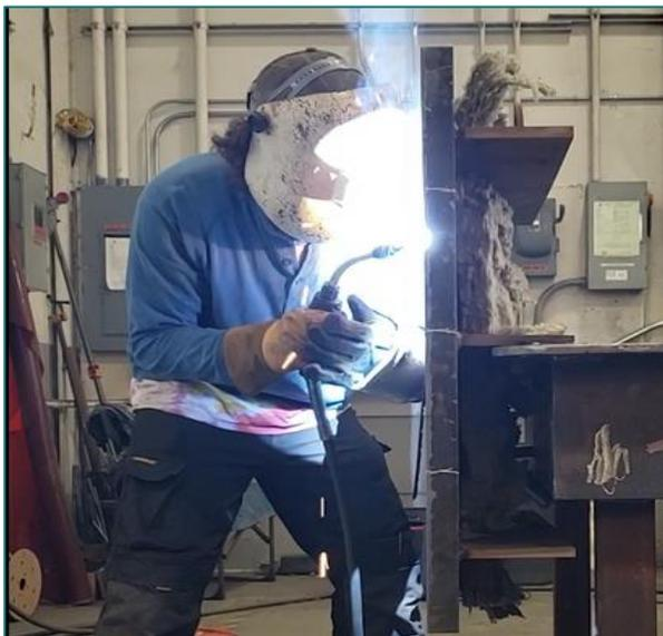
*Welding a Vertical Test Assembly*
