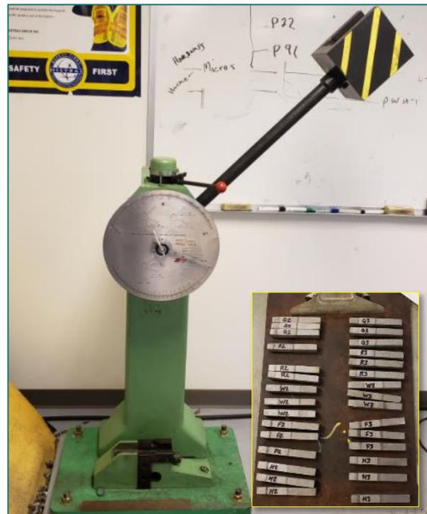
*Charpy V-Notch Test Machine and Coupons*
