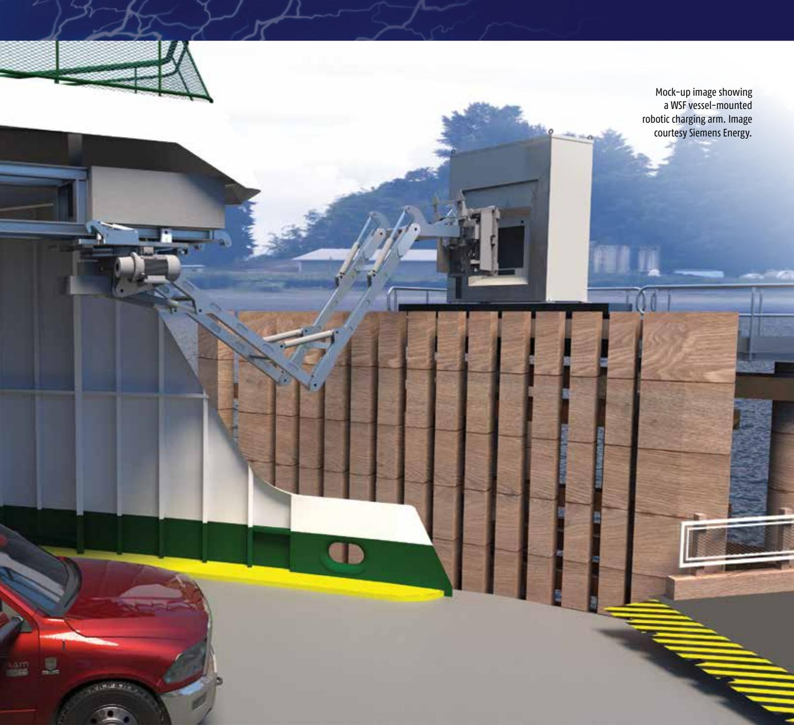
Mock-up image showing a WSF vessel-mounted robotic charging arm. Image courtesy Siemens Energy.
