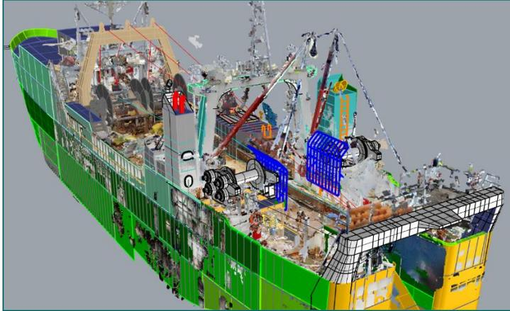
*3D model overlaid with vessel scan*
