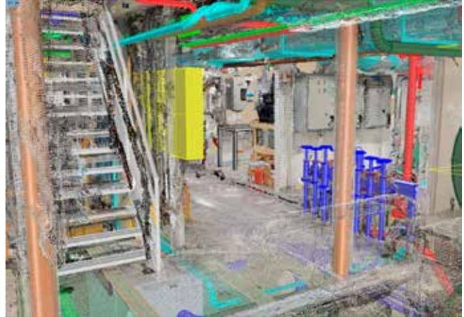
(LEFT) After construction, our engineers conducted a full vessel 3D scan using Matterport. This image of a point cloud shows the same engine room view as our model. (RIGHT) When we overlay the two images, scanned and model, we see the accurate details of construction to our design.
