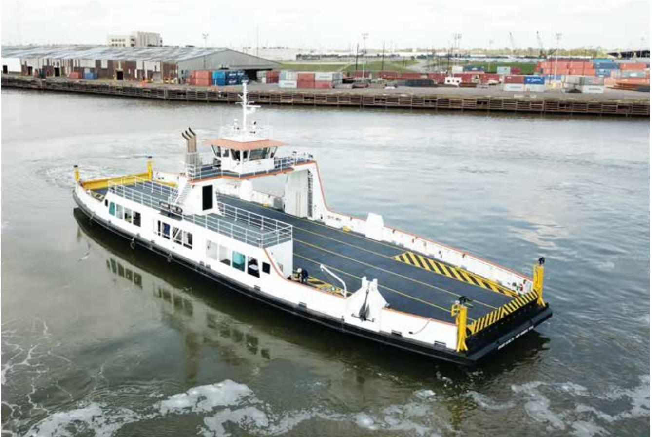
The EBDG designed diesel-electric *M/V Amadeo Saenz* owned and operated by the Texas Department of Transportation. EBDG performed a feasibility study for a possible conversion to hybrid diesel-electric propulsion. Photo courtesy of Travis Bergh, Southwest Shipyard.
