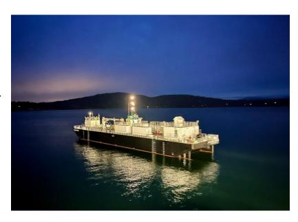
The barge is certified by the United States Coast Guard (USCG) for the recovery and disposal transport of petroleum products, ensuring compliance with applicable requirements outlined in USCG 46 CFR Subchapter D. Additionally, the vessel is classed by the American Bureau of Shipping (ABS) for Oil Spill Recovery.
